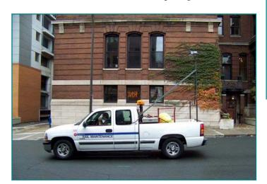
Engineers put a Hiawatha LRT horn and bell system on the back of a pickup to test noise impacts to Cedar Street buildings.
