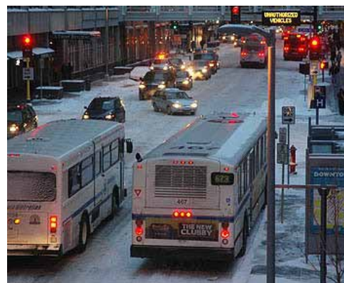
Double bus lanes on Second and Marquette avenues allow buses to pass each other, speeding up trips.
